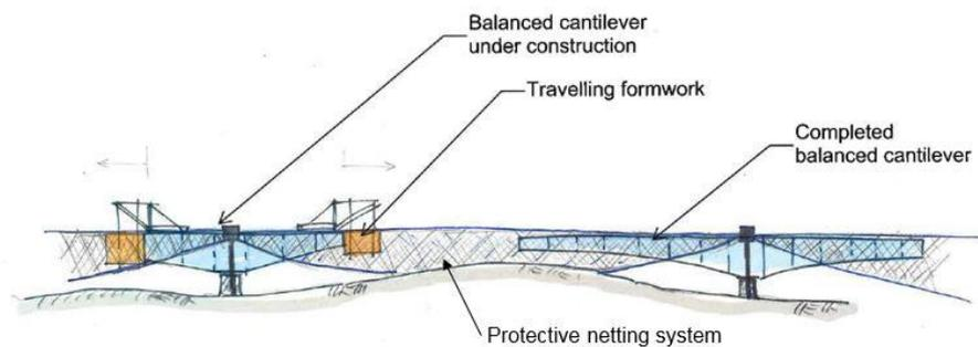
This is a less invasive construction methodology as it avoids any large scale construction works off the Limestone pavement, although, some parts of the bridge will be constructed using Construction Method 1. A netting system will also be used over the Limestone pavement and Turlough area to catch any falling debris or materials. This will ensure that no damage occurs to the Limestone pavement environment beneath.
